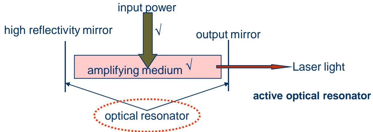
Optical resonator – cavity with reflecting walls, provides feedback of the electromagnetic field on discrete frequency, determines spatial distribution of the modes.
