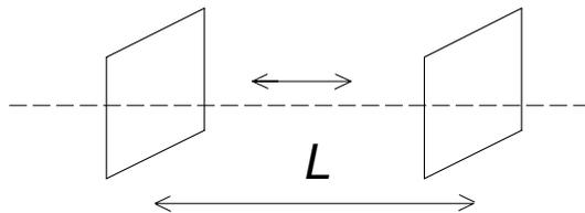
Superposition of two plane waves traveling in opposite directions along the cavity axis.
