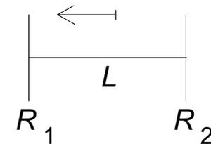
$$e^{-2\alpha_r L} = R_1 R_2 e^{-2\alpha_s L}, \quad \frac{1}{\alpha_r c} = \tau_r, \quad \boxed{\Delta\nu_r = \frac{1}{2\pi\tau_r}}, \quad \alpha_r = \frac{2\pi}{c} \Delta\nu_r.$$
