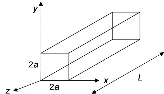
Removing side walls → open resonator,  $l, m \ll n$  (in practice 0, 1 or 2)
