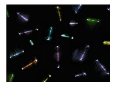
Multicolor nanowire lasers  $\emptyset$  200 - 400 nm, length 20 - 60  $\mu$ m Source: Optics & Laser Europe, August, 2008
