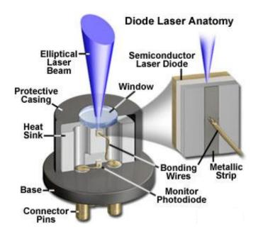
Laser diode 0.4 µm x 2 µm x 400 µm
