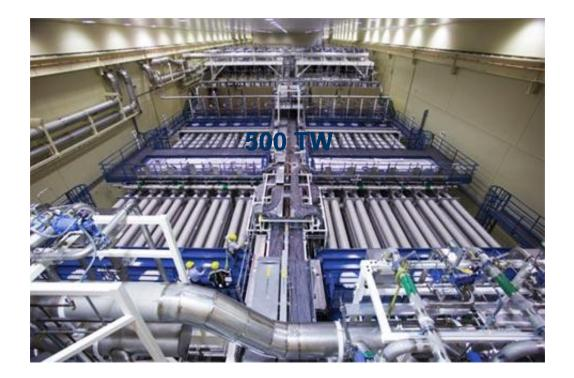
NIF, Lawrence Livermore National Laboratory, laser system with 192 beams: 500 TW, 7456 m laser
